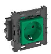
Protective contact socket with connection to side, Single 0°, with increased touch protection, with screwless terminals, 2-pin, 16 A, 250 V~, with connection terminals to IEC 60884-1, suitable for the installation in Rapid 80 device installation trunking system.
