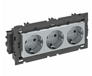
Protective contact socket with connection to side, triple 0°, with increased touch protection, with screwless terminals, 2-pin, 16 A, 250 V~, with connection terminals to IEC 60884-1, suitable for the installation in Rapid 80 device installation trunking systems.
