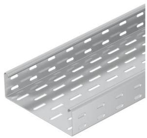
SKS 60 = Heavy-duty cable tray system with 60 mm side height. The cable tray, type SKS, should also be used for maintenance of electrical function. For additional data, please refer to BSS fire protection systems. The cable tray is fastened to the bracket with bolts, type FRS M6 x 12. Magnetic shield insulation without cover 20 dB, with cover 50 dB.
