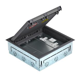
Square screed socket with GES9 UGE service outlet for use in screed floors for indoor use. With pre-marked insertion openings for pipelines (M25) on all four sides. With three cover plates. The minimum installation depth is 64 mm, the height-adjustment range +23 mm.
