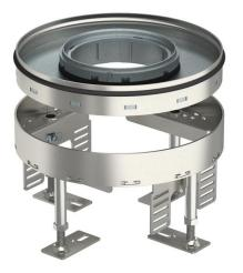
Round heavy-duty cassette for tube body of nominal size R4 for the installation of accessories in trunking systems, raised and cavity floors, in dry or wet-cleaned floors indoors. Load class 2 to 20 kN.
