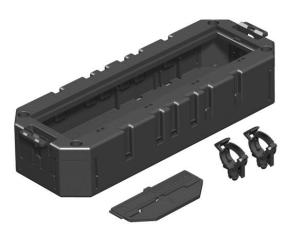
For the installation of up to 4 accessories of type Modul 45 in flush-mount units. Installation instead of a GB3 mounting box. The module support is closed in a downwards direction by two protective housings with a division 3+1 or 2+2. The scope of supply contains two strain reliefs and one separating retainer.
