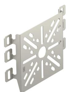
Mounting plate, for fastening on the side rail of cable support systems. Fastening on the side rail of the mesh cable tray is carried out without bolts by bending the lugs. Fastening on the side rail of cable trays or cable ladders is carried out with two truss-head bolts. Type B9/T junction boxes can be mounted very easily by inserting the bolt plug supplied into the centre hole on the mounting plate.
