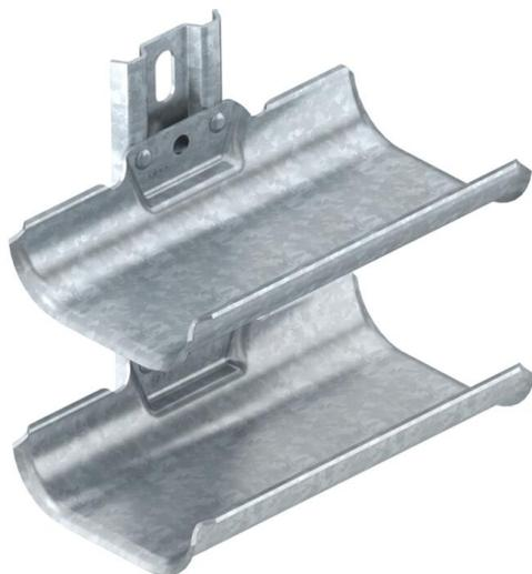
Cable support brackets for quick and easy routing of cables in areas where common cable support systems cannot be installed due to lack of space. The cable support brackets possess a large load-bearing surface as well as rounded outer edges to protect the cables. In accordance with DIN VDE 0298-300, a maximum support spacing of 0.8 m should not be exceeded.
