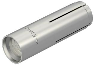
Drop-in anchor for single fixings of non-load-bearing systems in non-cracked concrete as well as for multiple fixings in cracked and non-cracked concrete.
