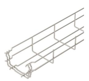
Mesh cable tray with shaped connector of side height 55 mm. No additional connection components are required for the mesh cable tray, it is simply interlocked. The grid width is 50 x 100 mm (exception: GRM 55/50 = 20 x  $^{\circ}$
