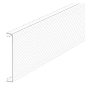
Trunking cover for closing Rapid 80 GK (PVC), GS (steel) and GA (aluminium) device installation trunking as well as ISS service poles with a 76.5 mm system opening. The GK-OTKKP cover is made from clear, transparent plastic and the inside is fluted (longitudinal) and is therefore suitable for integrating lighting in the trunking and service pole.
