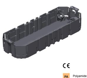
Empty mounting box with two strain reliefs for incoming and outgoing cables. Suitable for the installation of up to three standard or up to four Modul  $45^{\rm (I)}$  accessories in cover plates.
