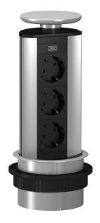
Lowerable Deskbox with connection cable for fixed installation on a tabletop, plastic fastening sleeve, painted accordingly in cover shade. It is mounted using a drill hole (Ø102 mm) in the tabletop.
