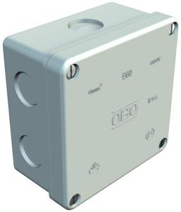
Protection rating IP54, rated voltage 660 V, nominal cross-section 6  $\div\,$  mm², two fastening holes for screws of up to 4.5 mm Ø in the interior of the box (seals and covers included), M6 fastening thread and adhesive area under the base, four
