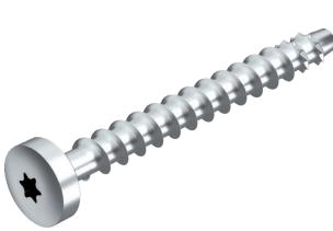
Bolt tie for direct mounting without additional anchors in cracked and uncracked concrete and masonry. With round head for universal fastenings. Torx drive T30.
