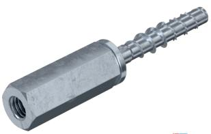
Bolt tie for direct mounting without additional anchors in cracked and uncracked concrete and masonry. With M8/M10 combination thread sleeve for fastening threaded rods.
