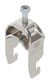
Clamp clip with U-foot, metal pressure sleeve with rounded edges to protect the cable. For vertical and horizontal mounting of 1 single cable on a C-profile rail. For slot width 18–22 mm. With 1-start screw thread on pressure sleeve, universal hexagonal screw head WAF10, with slot and cross recess. Suitable for assembly indoors and outdoors. We recommend the use of a counter-sleeve.
