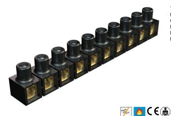
Terminals made of brass, screws of steel, galvanised and transparently passivated, 10-pole, strip separable into individual terminals, open on both sides. Captive upwards screw.
