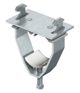
Clip element, bolt and lock plate made of hot-dip galvanised steel, pressure and counter-trough made of polypropylene, halogen-free, light grey RAL 7035.
